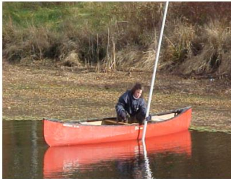
Figure M5.2: Measuring pond depth from canoe.
